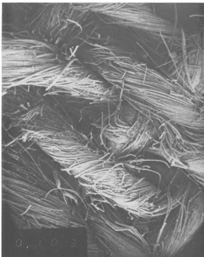
2. Scanning electron micrograph of the threads of the wrapping. Mag. \times 30
